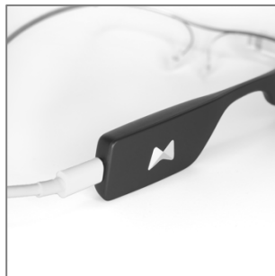
Figure 5- 2: Connecting the charging cable
