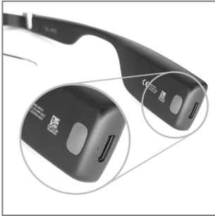
Figure 4- 3: Switching on the glasses
